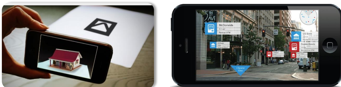
Figure 5: Examples of Image based AR and Location based AR. Images retrieved from https://thinkmobiles.com/blog/what-is-augmented-reality/
